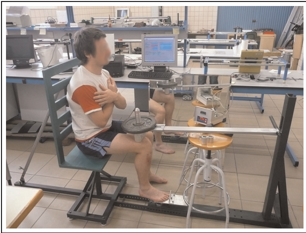
Figure 2. Global view of the experimental apparatus based on the measurement of lower leg vertical displacements.
